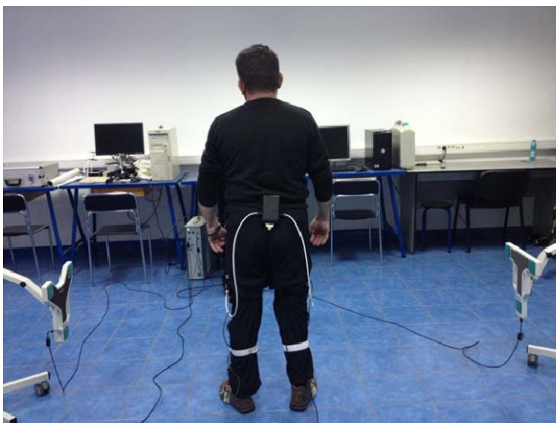
Fig. 1 The typical setup configuration of the gait analysis system.
