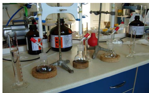
Fig. 2 Elution of column of activated Florisil ® Source: personal archive
