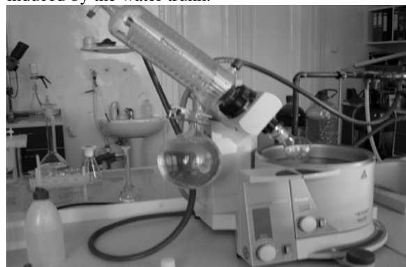
Fig. 1 The evaporation of the solvent in the extracted fat (source: personal archive)
