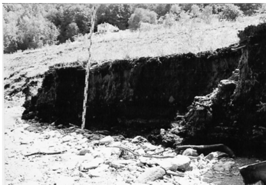
Fig. 9. The sediments deposits from Tarnița basin on the Someșul Cald branch. The thickness grow from the end of the retention towards the interior (0.30 m to 115 m and 1.21 m to 450 m distance) than they slowly reduce until the Someșul Rece II aqueduct outlet
